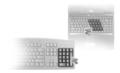
The numeric keypad functions like the numeric keypad on an external keyboard. Each key on the keypad has multiple functions. The keypad numbers and symbols are marked in blue on the right of the keypad keys. To type a number or symbol, press <Fn> and the desired key after enabling the keypad.
