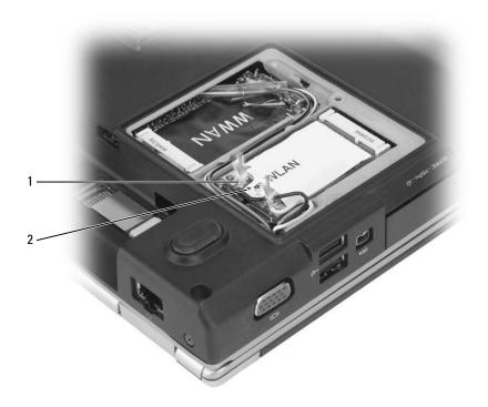
1 antenna cable connectors (2) 2 triangles (2)
