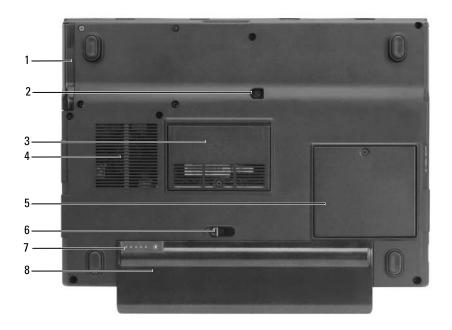
hard drive battery charge gauge air vents
